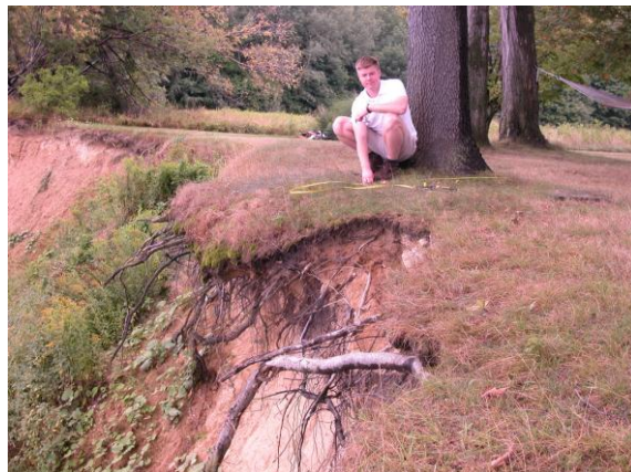
Figure 3: Measurement being taken to the bluff crest. In this case, the position of the bluff line is where the surveyor’s right arm is touching the ground – where the ground begins to break from the plane of the tableland – not at the edge of the growing grass.
