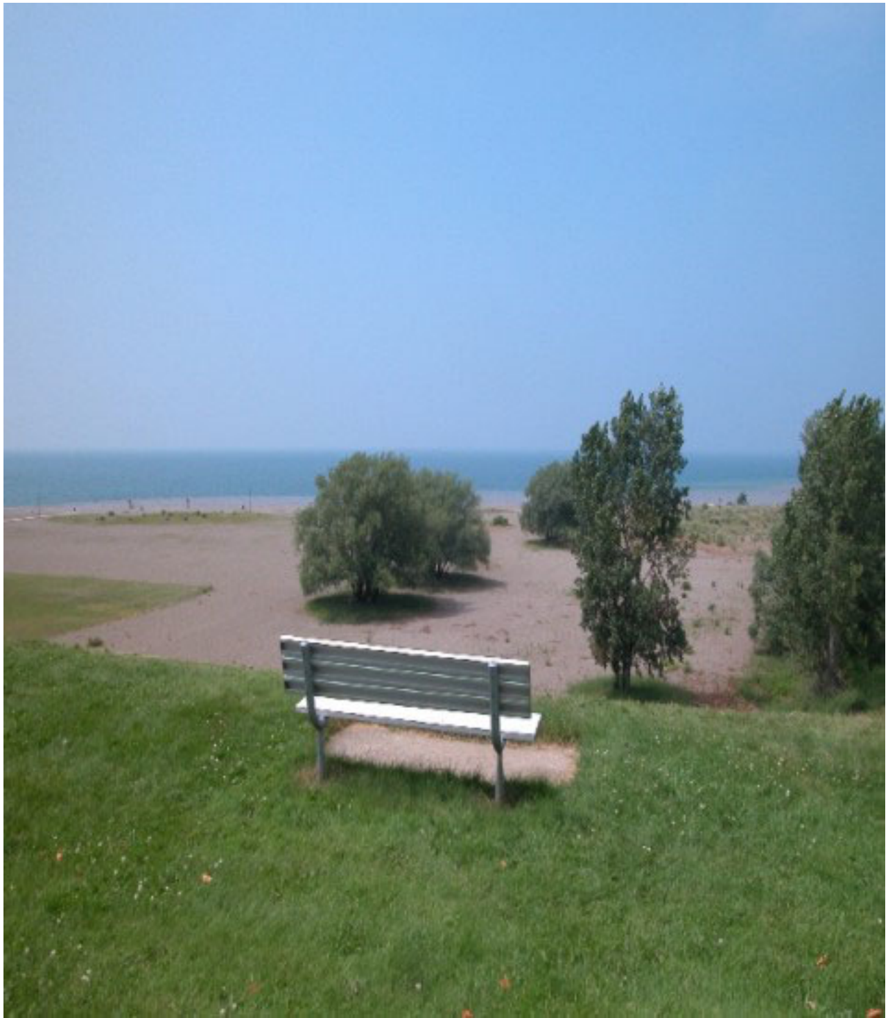
Figure #7 Date: 2005 Sand trapped by Conneaut Harbor's western harbor wall, which has created a very large sand fillet (beach) outside the harbor. Note: Bench is on a high bluff overlooking the sand fillet.
