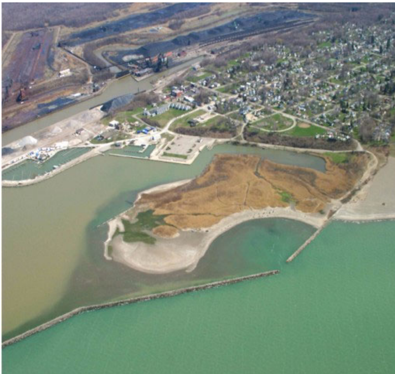
Figure #8 Date: April 19, 2006 Sand trapped inside Conneaut Harbor as a result of storm events washing littoral sand from the Conneaut fillet over the Harbor's western wall.
