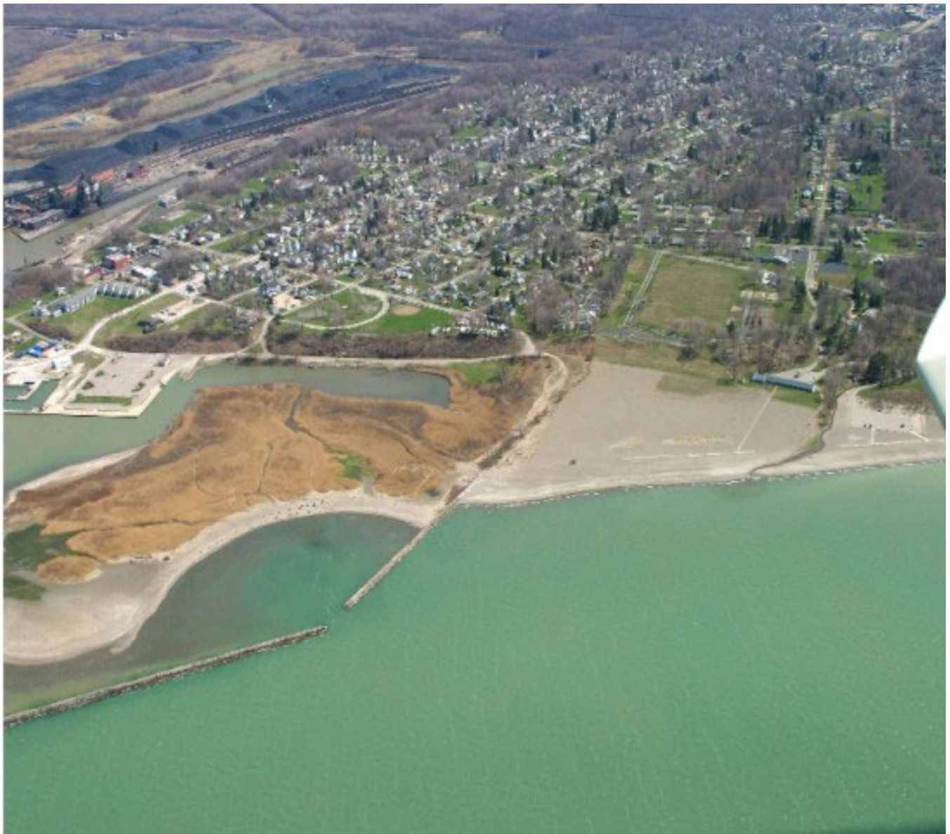
Figure #9 Aerial view of total amount of sand trapped by Conneaut Harbor.
