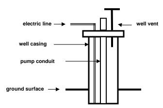
resistant screening. If the vent is not screened, it can become a potential entry point for debris and small animals. If concentrations in a vent pipe happen to exceed the lower explosive limit for methane (5 percent methane in air
