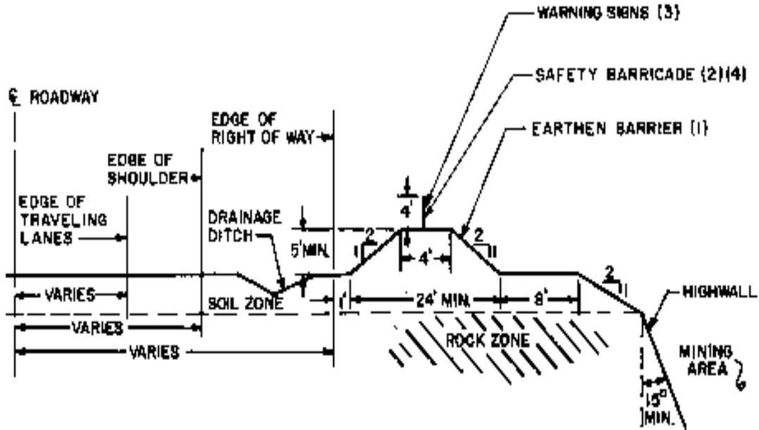
Figure 8-2: Using Natural Earthen Barrier (Compare to Figure 8.1)
