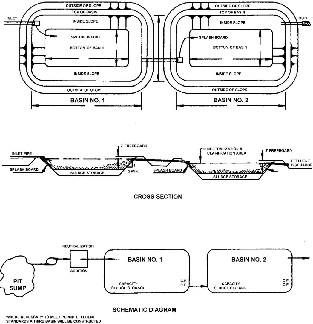
Figure 6-2: Typical Mine Drainage Neutralizer
