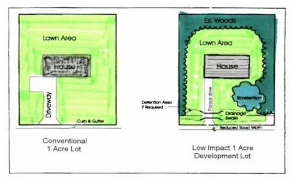
Figure 5.6-4 Convential Development Versus Low Impact Development
