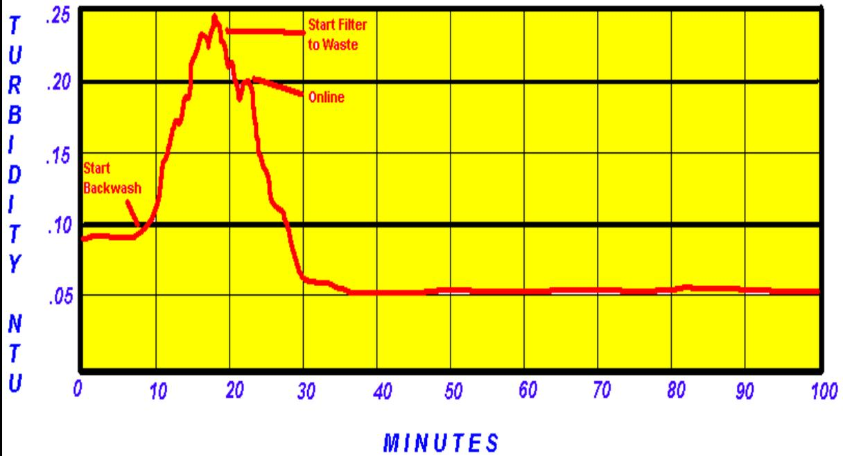
D.) *Secondary Spike: Increasing filter to waste probably won't eliminate this spike. Possible solutions may include increasing backwash rates and/or duration of backwash, or allowing filter to "rest" offline for at least 15 minutes before returning to service. Also, a plant may consider adding Alum to their backwash water during the last few minutes of the backwash sequence or adding a filter aid/polymer.*
