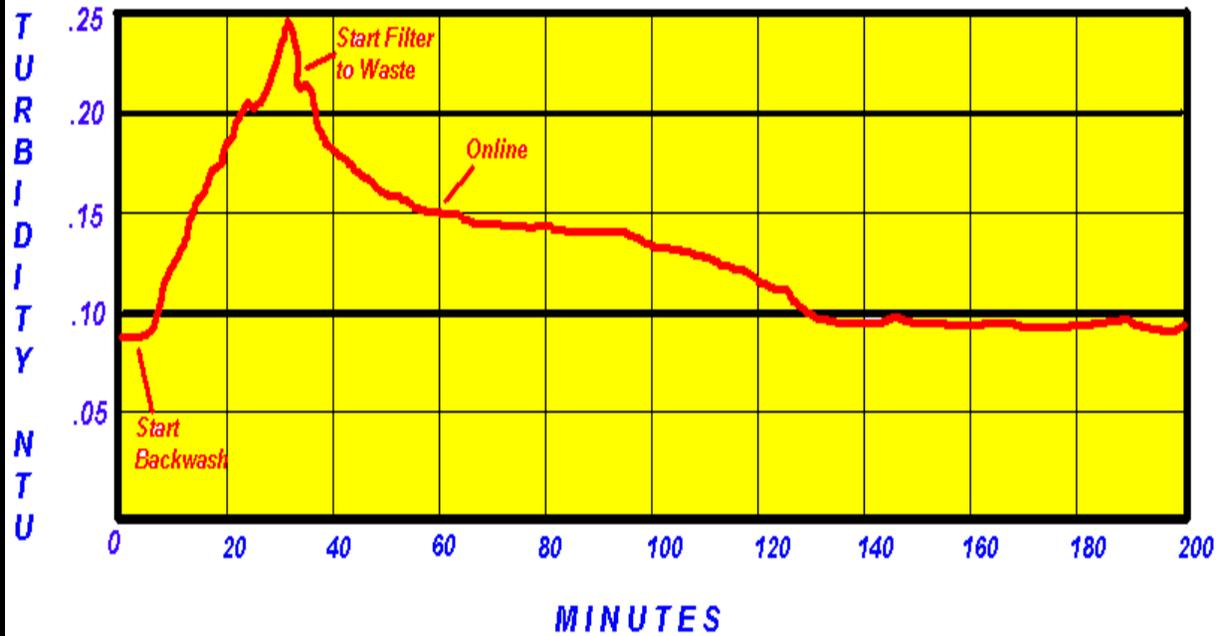
F.) Investigate similar causes as mentioned in Profile "E". However, this profile indicates that the filter appeared to be clean when returned to service, then breakthrough occurred quickly (in Profile "E" the filter never really recovered after backwashing). Sometimes, breakdown of a chemical feed pump may have caused this type of profile.
