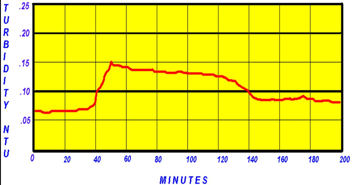
1.) This profile is caused by the start/stop operation of a plant. Filter to waste should be implemented whenever a "dirty" filter (filter with runtime) is placed online. Also, operating the plant at a lower flow rate would enable the plant to run longer with fewer shutdowns/startups and better overall process performance.
