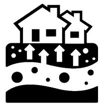
Radon is a naturally occurring radioactive gas produced by the breakdown of uranium in soil, rock, and water. Air pressure inside your home is usually lower than pressure in the soil around your home's foundation. Because of this difference in pressure, your house acts like a vacuum, drawing radon in through foundation cracks and other openings.
