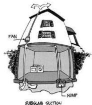
In houses that have a basement or a slab-on-grade foundation, radon is usually reduced by one of four types of soil suction:
