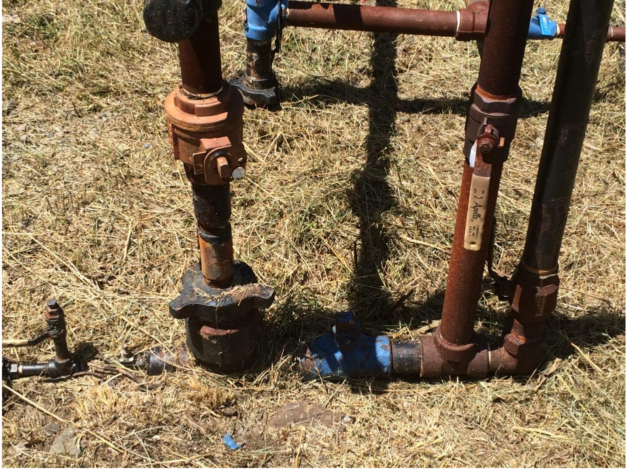
IMAGE 7. Photograph showing primary production annulus (8-5/8 inch by 4-1/2 inch) buried below surface with only tubing head exposed. Since no direct visual observation can be made, operator should record “inaccessible” instead of stating that no leaks are present.
