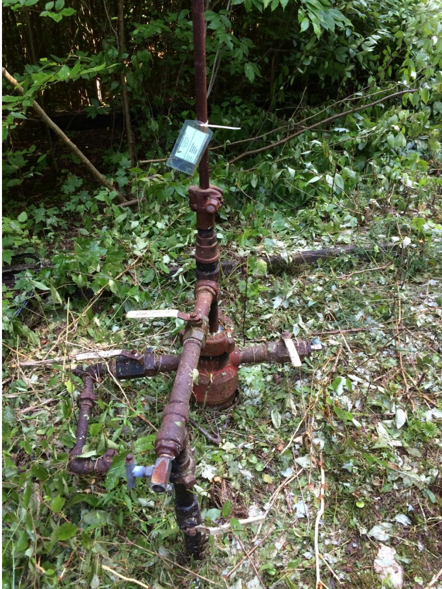
IMAGE 5. Photograph showing well at which operator reported 25 psi on 12/9/14. During the field verification study, the pressure was 0.5 psi inside the 7-inch by 2-inch annulus. The cups on the well are worn out and it is not cost effective to replace them according to the operator. It appears the well has not produced oil recently.
