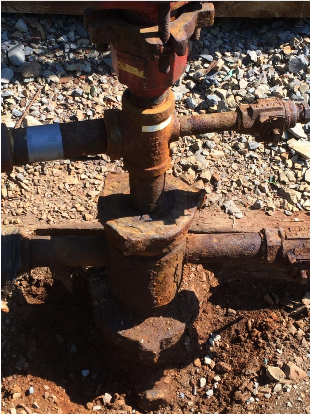
IMAGE 9. Photograph showing a well where operator reported production annulus pressure as 0 psig. Pressure could not be determined at the time of the field verification based on current well configuration. Operator should have reported that annulus was “inaccessible.” Severe corrosion was also noted but not reported by operator as part of Mechanical Integrity Assessment data submission.
