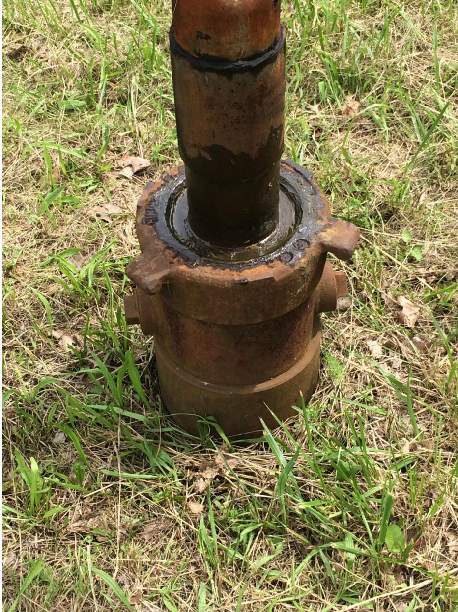
IMAGE 8. Photograph showing a well where operator reported production annulus pressure as 0 psig. Pressure could not be determined at the time of the field verification based on current well configuration. Operator should have reported that annulus was “inaccessible.”
