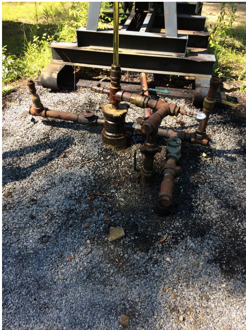
IMAGE 6. Photograph showing new gravel placed atop area of stained soil associated with stuffing box leaks. It appears the well is pumped fairly often as evidenced by the polished rod.
