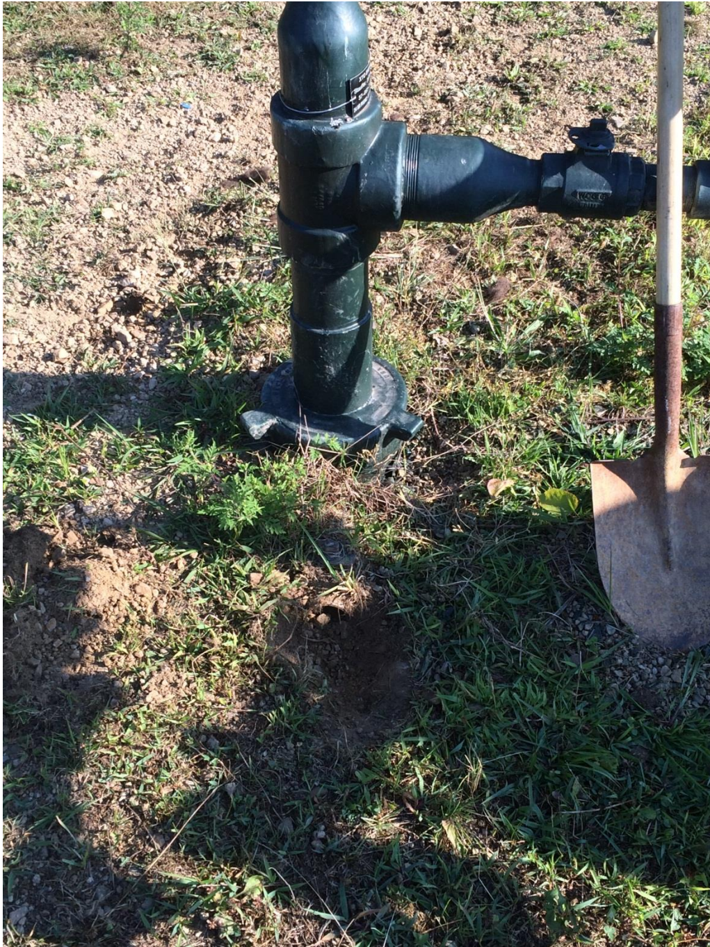
IMAGE 10. Photograph showing a well where operator reported production annulus as being vented. This may have resulted from an error in DEP computer coding for Forms A and B. For such a configuration, it is recommended that the operator use the comments field to indicate that the annulus is buried and report it as “inaccessible”.
